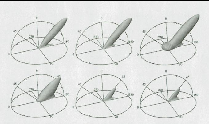
Fig. 16. Resampled scattering diagrams of the BRDF measurements of two paints: a blue enamel (top row) and a red automotive lacquer (bottom row). The RGB color measurements are shown from left to right.
