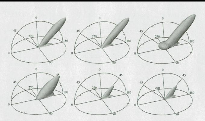
Fig. 16. Resampled scattering diagrams of the BRDF measurements of two paints: a blue enamel (top row) and a red automotive lacquer (bottom row). The RGB color measurements are shown from left to right.
