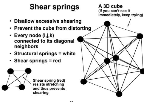
Shear spring (red) resists stretching and thus prevents shearing
