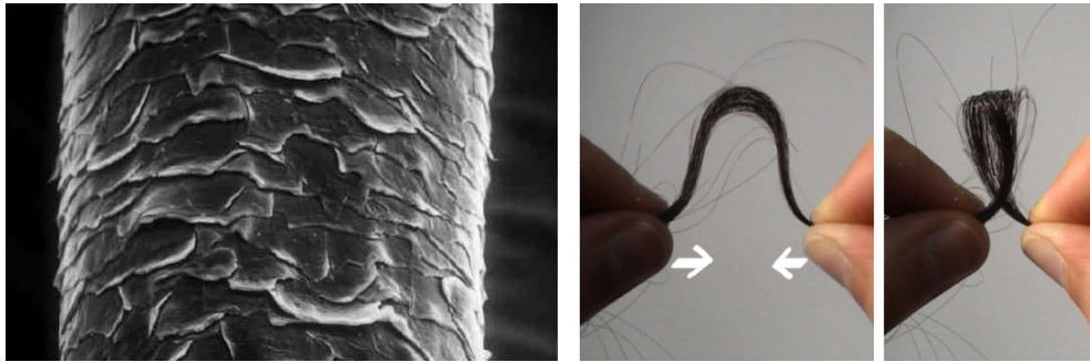
Figure 1.1: Left, close view of a hair fiber (root upwards) showing the cuticle covered by overlapping scales. Right, bending and twisting instabilities observed when compressing a small wisp.
