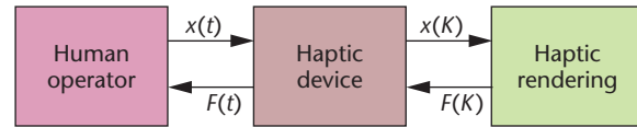
5 Haptic devices create a closed loop between user and haptic-rendering/simulation algorithms. x(t) and F(t) are continuous-time position and force signals exchanged between user and haptic device. x(K) and F(K) are discrete-time position and force signals exchanged between haptic device and virtual environment.
