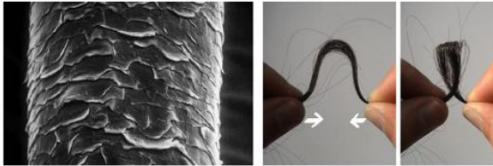
Figure 2: Left, close view of a hair fiber (root upwards) showing the cuticle covered by overlapping scales. Right, bending and twisting instabilities observed when compressing a small wisp.
