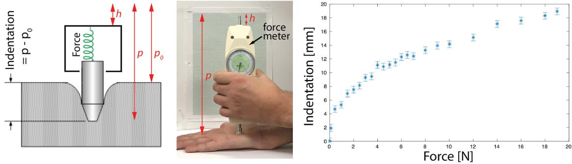
Figure 1: **Nonlinear durometer**: Left: Durometer schematics. Middle, right: We used our nonlinear durometer to measure the relationship between skin normal displacement and force, for the soft palm tissue. It can be seen that the relationship is very nonlinear. We also plot the confidence intervals, determined based on the precision of equipment used for this experiment.
