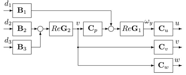
Fig. 1. Block diagram representation of the linearized 2D/3C model.
