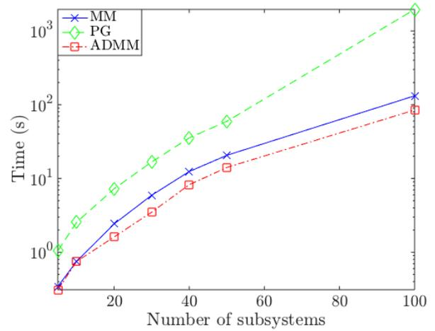
Fig. 2. Computation time required to solve (SP) for 10 evenly spaced values of  $\gamma$  from 0.001 to 1.0 for a mass-spring example with  $N = 5, 10, 20, 30, 40, 50, 100$  masses. Performance of direct proximal gradient (green dashed  $\diamond$ ), the method of multipliers (blue solid  $\times$ ) and ADMM (red dash-dot  $\square$ ) is displayed. All algorithms use BB step-size initialization.
