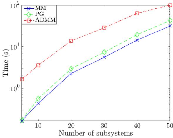
Fig. 3. Computation time required to solve (SP) for 20 evenly spaced values of  $\gamma$  from 0.001 to 0.05 for unstable network examples with  $N = 5, 10, 20, 30, 40, 50$  nodes. Performance of direct proximal gradient (green dashed  $\diamond$ ), the method of multipliers (blue solid  $\times$ ) and ADMM (red dash-dot  $\square$ ) is displayed. All algorithms use BB step-size initialization.
