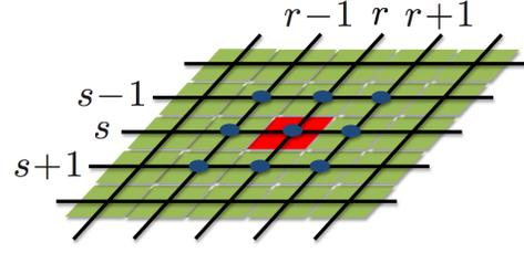
Fig. 2. Sketch of a localized control strategy where the actuator placed at  $(r, s)$  uses information from only the nearest neighbors on the lattice.
