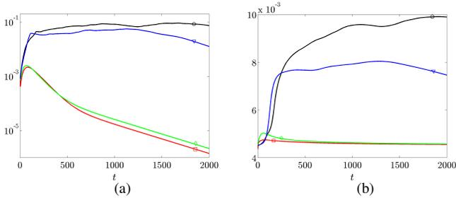
Fig. 4. (a) Energy of the velocity fluctuations  $E(t)$ ; and (b) skin-friction drag coefficient  $C_f(t)$  for the flow with no control ( $\circ$ ) and centralized ( $\square$ ), truncated centralized ( $\nabla$ ), and localized ( $\diamond$ ) controllers. The results are obtained using direct numerical simulations with  $R_c = 2000$ .
