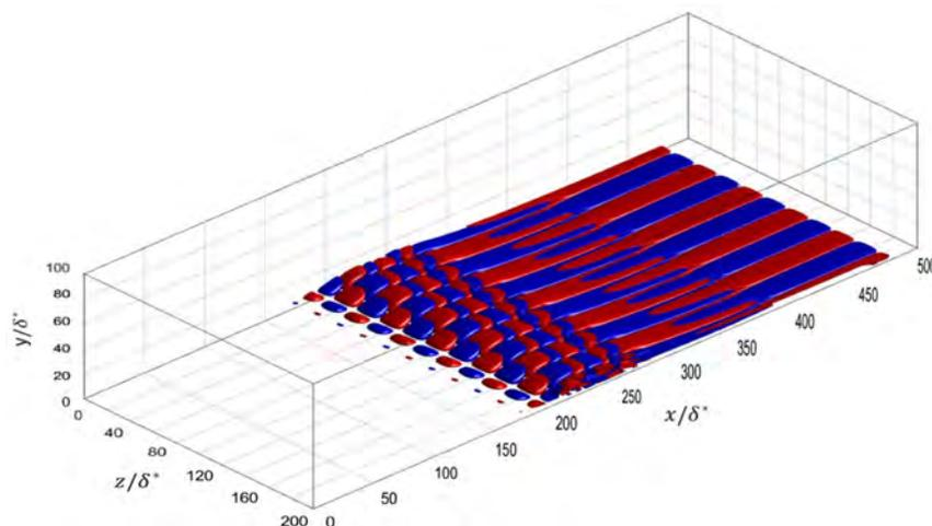
**Figure 16: The most unstable mode in Figure 15 visualized by the real part of the normalized streamwise velocity perturbation. Here red denotes a positive velocity while blue is negative.**
