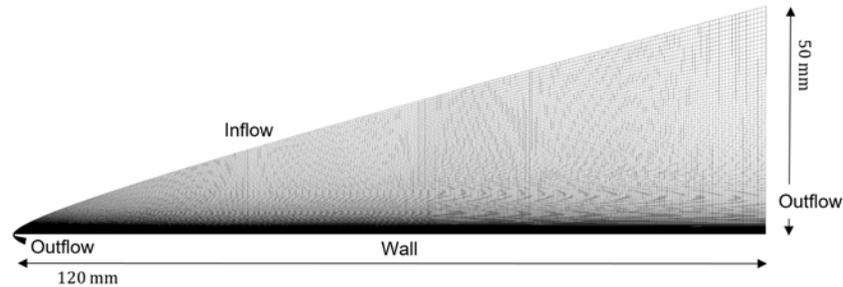
Figure 17: Stretched grid used for the 2D calculation of the incoming boundary layer.
