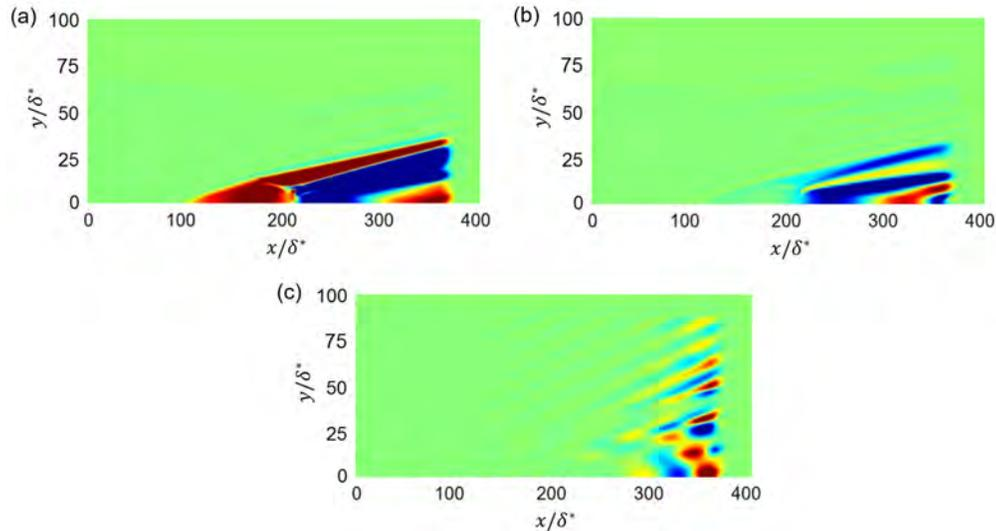
**Figure 14: Global modes corresponding to labels in Figure 13 colored with the real part of the pressure perturbation. Here red denotes a positive pressure while blue is negative.**
